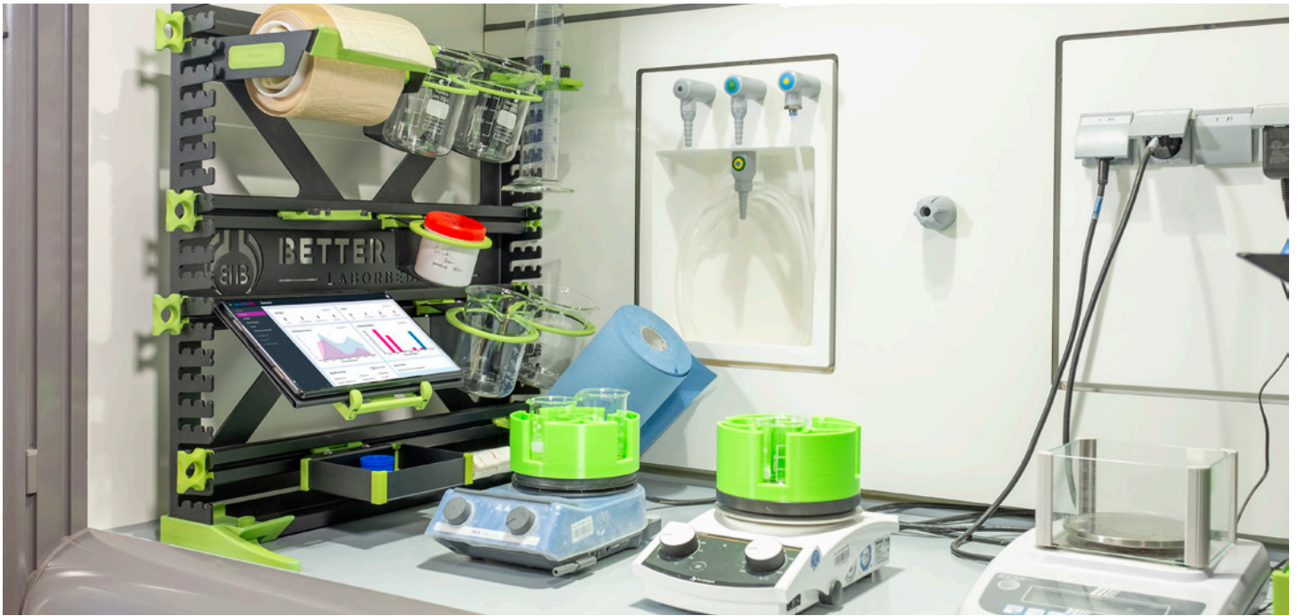
Storage boxes and holders in the SmartRack® allow quick access to lab vessels and support efficient workflows in the fume hood.
