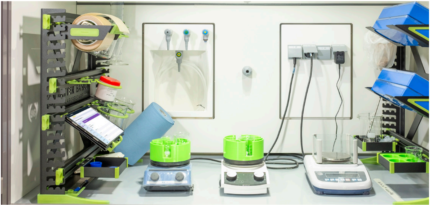
The SmartRack® provides structured storage, digital documentation, and efficient use of limited space inside the laboratory fume hood.
